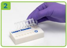
Remove one test strip and one diluent tube from the packaging. Place the diluent tube and test strip in the rack provided, ensuring that the blue tube goes into the recess with a blue circle around it. Put the remaining tests back into the fridge immediately.
