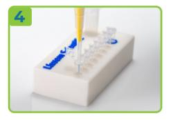
Using a new pipette tip, transfer 5  $\mu$ l of the mixed liquid from the diluent tube into the first tube of the test strip. Use the pipette to mix well.
