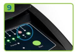
The positive control in tube 7 should always be **positive** and the negative control in tube 8 should always be **negative**. This indicates the test QC has passed and the results can be accepted. If either control fails, refer to the Troubleshooting Guide.
