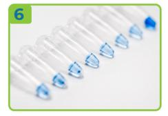
Once complete, all tubes should have equal volume and be a uniform blue. All liquid should be at the bottom of the tubes, with no air bubbles. Gently flick the tubes to remove any air bubbles.
