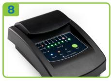
A red LED indicates a 'positive' result and a green LED indicates a 'negative' result. If more than one bacterial tube is positive, this could indicate a mixed infection.
