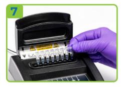
The test should now be run immediately. Place the test strip into the Lodestar DX analyser ensuring that the tube hinges are facing backwards and to the right.
