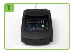
Switch on the Lodestar DX analyser. When the 'Ready' light is bright green, you can start to prepare the test.
